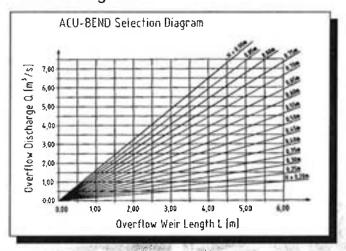
The calculation of the overflow discharge Q is based on the Poleni weir formula
