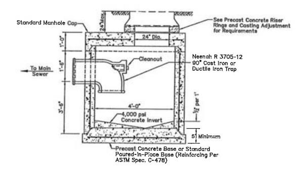
Note: General Construction Requirements Same as Standard 48" Manhole Structure Base Alternatives Same as Standard 48" Manhole
