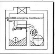
Diagram arrangement in combination with an ACU-BEND overflow bending weir H
