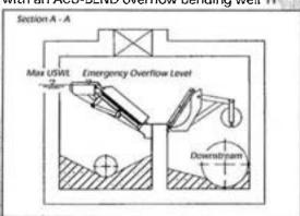
Vertical arrangement with auxiliary sill and screened material storage chamber
