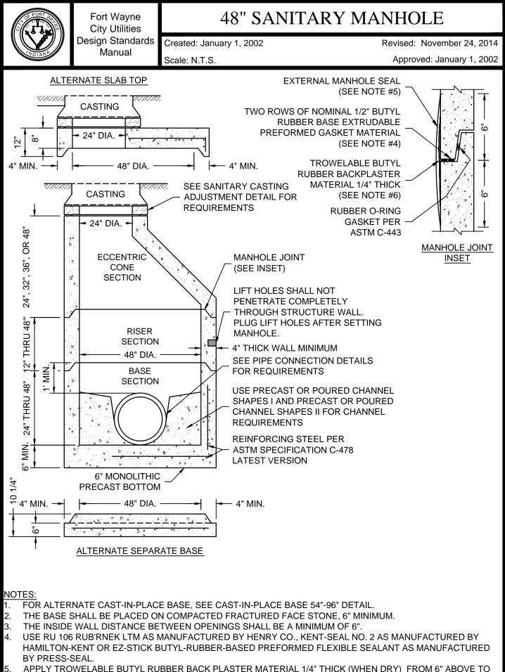
APPLY TROWELABLE BUTYL RUBBER BACK PLASTER MATERIAL 1/4" THICK (WHEN DRY) FROM 6" ABOVE TO 6" BELOW JOINTS. USE TROWELABLE EZ-STICK #3, AS MANUFACUTRED BY PRESS-SEAL GASKET CORP.
