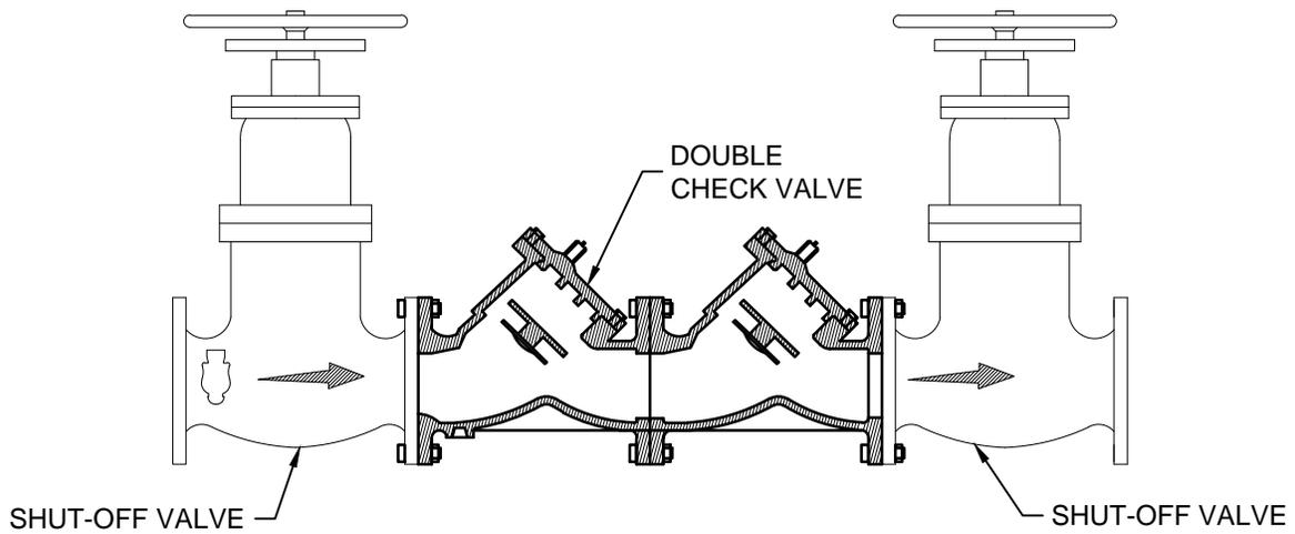
TYPICAL ARRANGEMENT OF DOUBLE CHECK VALVE
