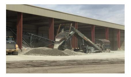
The BHF is equipped to reclaim spoils and process into road bed clay for lagoon repair and flood control. Top soil from spoils is used for restoration work.
