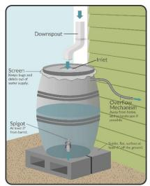
goal is to prevent pooling of water around the base of the rain barrel. If you have a rain garden, this is a good place to divert the excess water.
