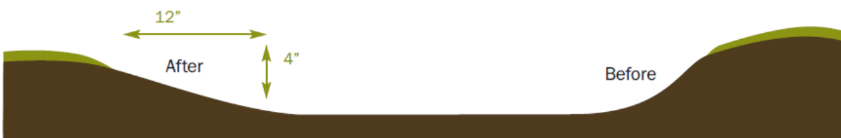
Figure 6: Sloping the sides of a Rain Garden
